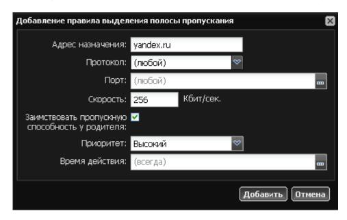
By ticking the option "reserve bandwidth from parent", traffic defined in the rule can use more bandwidth than specified in the rule if the internet channel is free.
